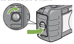
When loading the SD Memory Card, take care not to get any dirt on the card's metal parts.
