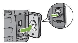
4 Open the terminal cover, and then connect the USB cable to its USB terminal.
