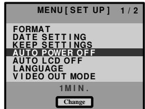
**3 Press the MENU  button and select the setting time (1 MIN, 3 MIN, 5 MIN, OFF)**
