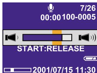
Press the ▲ or ▼ button during playback to display the volume indicator. Press the ▲ or ▼ button to adjust the volume.
