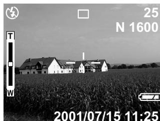
The zoom indication bar will be displayed on the LCD monitor. Adjust the subject to the desired size.
