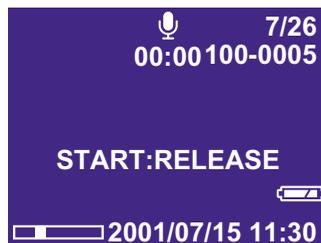
The voice memo will be played back and the playback indicator and time elapsed will be displayed. Playback of voice memo files ends automatically. During playback, you can rewind the voice memo file with the ◀ button, and fast forward with the ▶ button.
