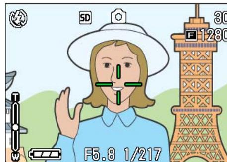
Once the shot is in focus, the exposure and white balance are fixed and the crosshair in the center of the LCD Monitor turns green, as does the auto-focus lamp in the lower left of the Viewfinder. Check one of these to make sure the subject is in focus.
