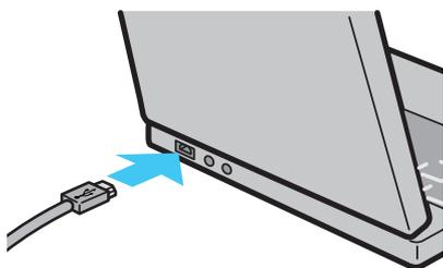
3. Open the terminal cover, and then connect the USB cable to its USB terminal.
