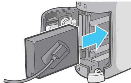
4. **Open the power (DC input) cable cover and take the cable out.**
