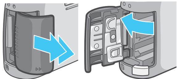
3. **Insert the two batteries, making sure they are facing the correct way..**
