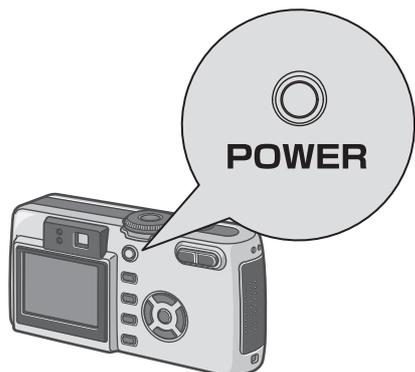
After the start sound, the flash lamp and auto-focus lamp blink alternately for several seconds.
