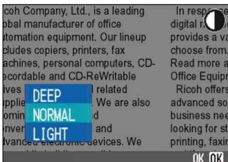
4. Press the ▲▼ buttons to select the desired density setting.
