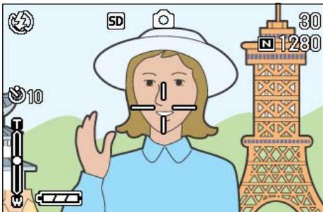
The Self Timer mark appears momentarily in a large size at the center of the LCD monitor and then is displayed at the upper left.
