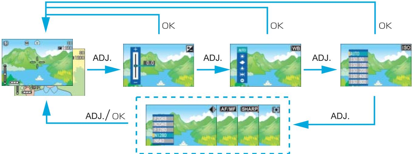
Use the SETUP screen to register a function to the ADJ button.
