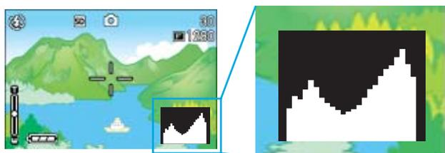
A histogram is a graph indicating the number of pixels on the vertical axis and the brightness on the horizontal axis. The brightness is shadow (dark), halftone, and highlight (light) from the left.
