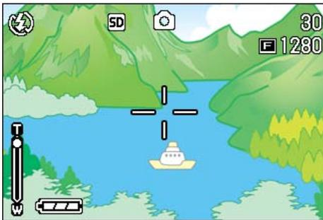
3. With the subject image enlarged to the end of the T side (Telephoto) on the Zoom Bar, release the [A] button once and press [A] button again and hold down.
