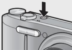
If the POWER button is pressed when the camera is on, the number of files recorded on that day is displayed, and then the camera turns off.
