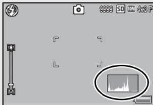
By using the histogram, you can determine the brightness of an image without being affected by the brightness around the picture display. This also helps you correct for areas that are overly bright or dark.
