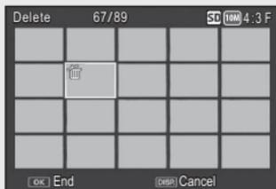
**4** Press the ADJ./OK button ▲▼🗑️⚡ to select the ending point of the range of files you want to delete and press the ADJ./OK button.
