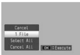
To add a photo to or remove it from the print order, select [1 File] and press the ADJ./OK button
