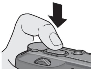
**If the camera is unable to focus**, the center focus frame blinks red and the autofocus/flash lamp blinks green.
