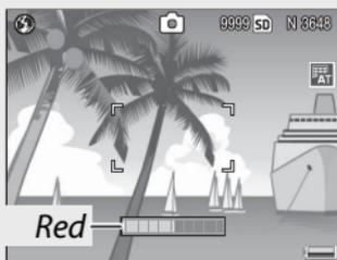
Unable to measure tilt; camera rotated too far forward or back
