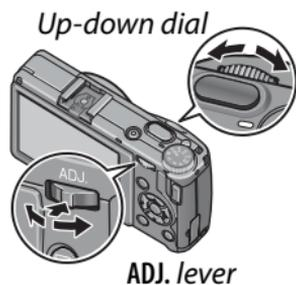
You can assign frequently-used shooting menu items to the ADJ. lever for easy access. To display a shooting menu item, center the ADJ. lever and press it in; you can then use the lever and up-down dial to select an option as described on page 116.
