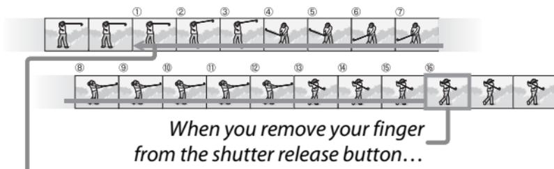
...the camera records the frames taken in the last two seconds (frames ① to ⑯).
