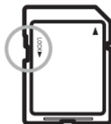
Pictures can not be taken when the memory card is locked; lock the card only to prevent accidental loss of data and be sure to unlock the card before shooting.
