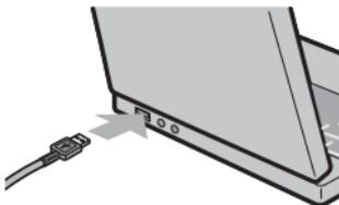
Connect the cable to the camera as shown. The camera will turn on, DL-10 will start, and transfer will begin automatically. Pictures are copied to folders in the "Digital Camera" folder in "My Documents" (if you were previously using Caplio software, pictures will instead be copied to folders in the "Caplio" folder). Pictures are sorted into separate folders by date of recording; make sure the camera clock is set to the correct date and time before shooting.
