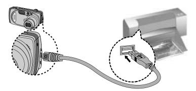
% If [COMPUTER] is selected at step 5, the camera will not connect to the printer, and the autofocus lamp will just blink green.
