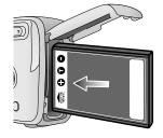
2. Insert the batteries taking note of the polarity (+ / -).
