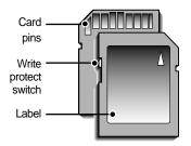
The SD memory card has a write protect switch that prevents image files from being deleted or formatted. By sliding the switch to the bottom of the SD memory card, the data will be protected. By sliding the switch to the top of the SD memory card, the data protection will be canceled. Slide the switch to the top of the SD memory card before taking a picture.
