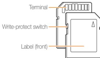
You can prevent files from being deleted by using the write-protect switch on the SD or SDHC card. Slide the switch down to lock or slide it up to unlock. Unlock the card when shooting.
