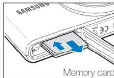
Push the card gently until the card disengages from the camera, and then pull it out of the slot.
