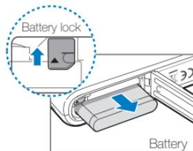
Push the lock up to release the battery.
