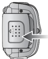
2. Have the front of the memory card facing toward the back of the camera (LCD monitor) and the card pins toward the front of the camera (lens), and then push the memory card into the card slot until you hear a click.
