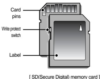
The SD memory card has a write protect switch that prevents image files from being deleted or formatted.
