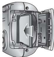
3. To close, push the battery chamber cover until you hear a click. If the memory card does not slide in smoothly, do not attempt to insert it by force. Check the direction of insertion, and then insert it correctly. Do not insert the memory card the wrong way round. Doing so may damage the memory card slot.
