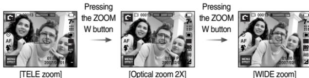
**Digital zoom WIDE** : When the digital zoom is in operation, pressing the ZOOM W button will reduce the digital zooming in steps. Releasing ZOOM W button stops digital zooming. Pressing the ZOOM W button will reduce the digital zoom and then it will continue to reduce the optical zoom until the minimum setting is reached.
