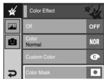
Press the OK icon and the Mask mark will display on the LCD monitor
