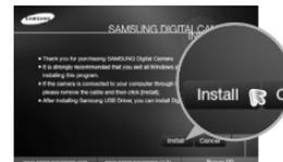
2. Install the camera driver and DirectX by selecting a button shown on the monitor.
