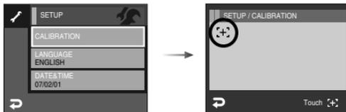
※ When you calibrate the LCD monitor, press the Calibration point exactly or menus on the LCD monitor aren't selected or set.
