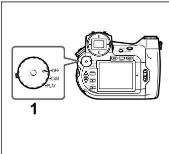
**1** Make sure the camera power/mode dial is set to the OFF position.
