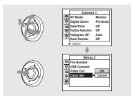
To change the current settings of the camera, bring up the menu or the SET UP screen (pages 47, 48), and use the multiselector to make the changes.
