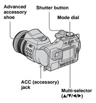
When an external flash is mounted, the weight prevents the lens portion from becoming steady.
