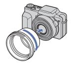
2 Position the lens hood as shown below and turn the lens hood clockwise until it clicks.
