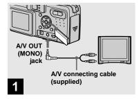
Connect the supplied A/V connecting cable to the A/V OUT (MONO) jack of the camera and the audio/video input jacks of the TV.
