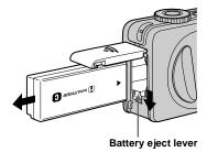
Open the battery/"Memory Stick" cover. Slide the battery eject lever in the direction of the arrow, and remove the battery pack.
