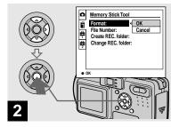
Select (Memory Stick Tool) with △/▼ on the control button. Select [Format] with ▶, then press ▶. Select [OK] with △, then press ●.
