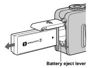
Open the battery/"Memory Stick" cover, and push down the battery eject lever in the arrow direction as illustrated above.
