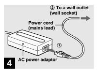
Connect the power cord (mains lead) to the AC power adaptor and to a wall outlet (wall socket).
