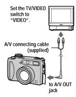
Connect the A/V connecting cable to the A/V OUT jack of your camera and to the audio/video input jacks of the TV.
