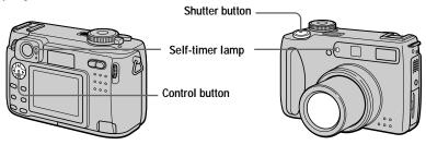
Clear the menu (page 41), then press the control button  $\nabla$  ( $\otimes$ ). The  $\otimes$  (self-timer) indicator appears on the LCD screen, and about 10 seconds after you press the shutter button, the subject is recorded. The self-timer lamp flashes and the beep sounds after you press the shutter button until the shutter is released. To cancel the self-timer recording, press the control button  $\nabla$  ( $\otimes$ ) again.
