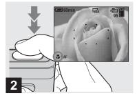
Center the subject in the frame. Press and hold the shutter button halfway down, then press the shutter button fully down.
