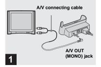
➡ Connect the A/V connecting cable (supplied) to the A/V OUT (MONO) jack of the USB cradle (supplied) and the audio/video input jacks of the TV.
