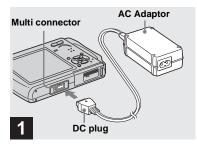
Connect the AC Adaptor (supplied) to the multi connector of the camera.
