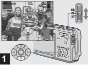
Set the mode switch to ☐, and press ▼ (⑤) on the control
