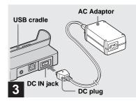
→ Connect the AC Adaptor (supplied) to the DC IN jack of the USB cradle (supplied).
