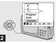
Select ▲ (Camera) with ◄ on the control button, then select the desired mode with ▲/▼.
