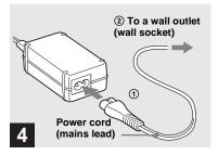
Connect the power cord (mains lead) to the AC Adaptor and to a wall outlet (wall socket).
