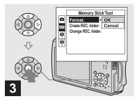
→ Select (Memory Stick Tool) with ▲/▼ on the control button. Select [Format] with ▶, then press ▶.
