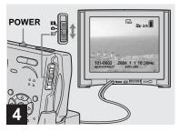
→ Set the mode switch to ▶, and turn on the camera.
