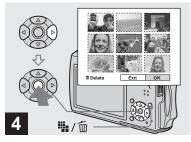
➡ Press 11/m (Delete) and select [OK] with ▶ on the control button, then press •.
