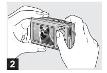
Hold the camera steadily with both hands and position the subject in the center of the focus frame.
