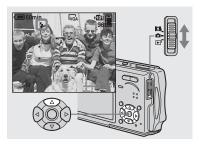
Set the mode switch to ☐, and press ▲ (≵) on the control button repeatedly to select a flash mode.
