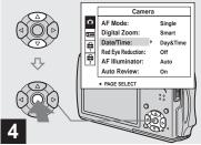
Select the date and time setting with ▲/▼ on the control button, then press ●.
