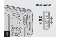
→ Set the mode switch to ▲, and turn on the power.
