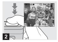
➡ Center the subject in the frame. Press and hold the shutter button halfway down, then press the shutter button fully down.
