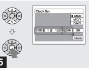
→ Set the numeric value with ▲/▼ on the control button, then press ● to enter it.
