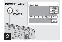
Press the POWER button to turn on the camera.
