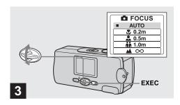
→ Select the desired focus setting with A/▼ on the control button, then press EXEC.
