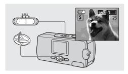
→ Set the mode switch to STILL, and press ▲ (‡) on the control button repeatedly to select a flash mode. Each time you press  $\blacktriangle$  ( $\clubsuit$ ), the indicator changes as follows:
