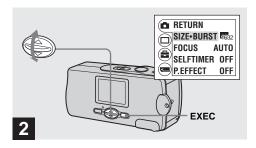
→ Select [n] with A/V on the control button, then press EXEC. Select [SIZE-BURST] with A/V on the control button, then press EXEC.
