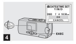
Select [OK] with ▲/▼ on the control button, then press EXEC.
