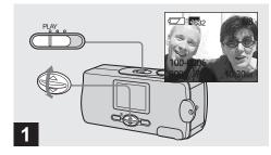
⇒ Set the mode switch to PLAY, and display the image you want to print with △/▼ on the control button.
