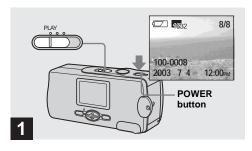
Set the mode switch to PLAY, and press the POWER button to turn on the power.
