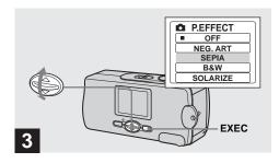
→ Select the desired mode with A/▼ on the control button, then press EXEC.
