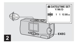
→ Select the desired date display format with A/▼ on the control button, then press EXEC.
