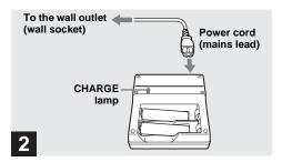
Connect the charger to a wall outlet (wall socket) using the power cord (mains lead).
