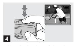
Press the shutter button halfway down, then hold the shutter button fully down.
