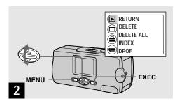
→ Press MENU and select [▶] with ▲/▼ on the control button, then press EXEC.
