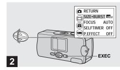
→ Select [♠] with ▲/▼ on the control button, then press EXEC. Select [SIZE-BURST] with ▲/▼ on the control button, then press EXEC.
