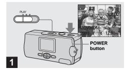
Set the mode switch to PLAY, and press the POWER button to turn on the power.
