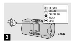
→ Select [DELETE] with A/▼ on the control button, then press EXEC.
