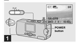
→ Set the mode switch to PLAY, and press the POWER button to turn on the power. Press ▲/▼ on the control button to select the image you want to delete.
