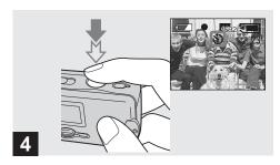
Center the subject in the LCD screen, and press and hold the shutter button halfway down.
