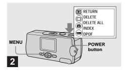
Press the POWER button to turn on the power, and press MENU.
