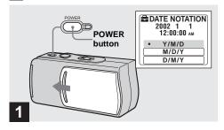
→ Slide the lens cover in the direction of the arrow or press the POWER button to turn on the power.
