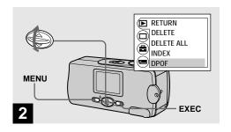
→ Press MENU, and select [▶] with ▲/▼ on the control button, then press EXEC. Select [DPOF] with ▲/▼ on the control button, then press EXEC.
