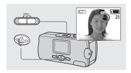
→ Set the mode switch to STILL, and press ▼ (SCENE) on the control button repeatedly to select a desired mode. Each time you press ▼ (SCENE), the indicator changes as follows:
