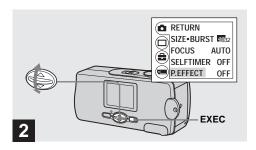
→ Select [n] with A/▼ on the control button, then press EXEC. Select [P.EFFECT] with A/▼ on the control button, then press EXEC.
