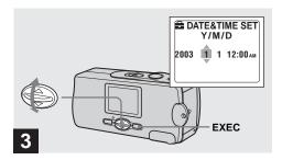
→ Set the numeric value with A/▼ on the control button, then press EXEC.
