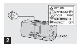
→ Select [ ] with A/▼ on the control button, then press EXEC. Select [SELFTIMER] with A/▼ on the control button, then press EXEC.
