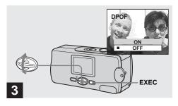
Select [ON] with ▲/▼ on the control button, then press EXEC.
