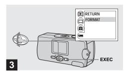
→ Select [ with A/ on the control button, then press EXEC. Select [FORMAT] with A/ on the control button, then press EXEC.
