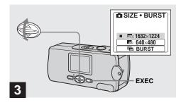
→ Select the desired image size with A/▼ on the control button, then press EXEC.
