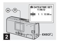
→ Select the desired date display format with the control buttons ▲/▼, then press EXEC.
