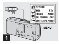
→ Set the mode switch to 間, and open the lens cover to turn on the power.
