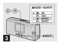
→ Select [♠ BURST] or [♠ BURST] with the control buttons ▲/▼, then press EXEC.
