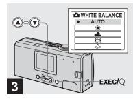
→ Select the desired mode with the control buttons ▲/▼, then press EXEC.
