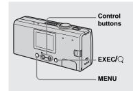
To change the current settings of the camera, bring up the menu, and use the control buttons to make the changes. For each item, press MENU to display the menu and press the control buttons  $\blacktriangle/\blacktriangledown$  to select the desired value, then press EXEC to make the setting.
