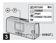
Select [ ] with the control button ▼, then press EXEC. Select [FORMAT] with the control buttons ▲/▼, then press EXEC.
