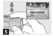
→ To stop recording, press the shutter button fully again.
