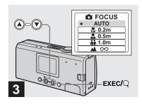
→ Select the desired focus setting with the control buttons ▲/▼, then press EXEC.
