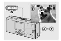
→ Set the mode switch to □, and press the control button ▲ (‡) repeatedly to select a flash mode.
