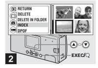
⇒ Select [▶] with the control button ▲, then press EXEC. Select [INDEX] with the control buttons ▲/▼, then press EXEC.
