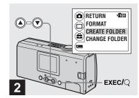
→ Select [ ] with the control button ▼, then press EXEC. Select [CREATE FOLDER] with the control buttons △/▼, then press EXEC.
