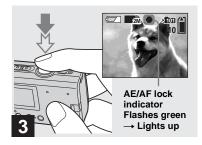
Press and hold the shutter button halfway down.
