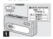
→ Slide the lens cover in the direction of the arrow or press POWER to turn on the power.
