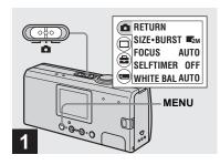
→ Set the mode switch to □, and turn on the power, then press MENU.
