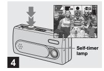
Center the subject in the LCD screen and press the shutter button fully down.
