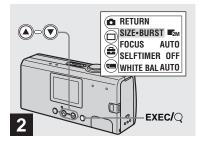
→ Select [♠] with the control button ♠, then press EXEC. Select [SIZE-BURST] with the control buttons ♠/▼, then press EXEC.
