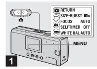
Set the mode switch to , and turn on the power, then press MENU.
