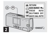
→ Select [n] with the control button A, then press EXEC. Select [SIZE-BURST] with the control buttons A/▼, then press EXEC.
