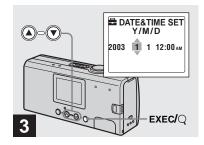
Set the numeric value with the control buttons ▲/▼, then press EXEC.
