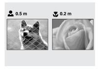
When shooting an image using a previously set distance to the subject, or when shooting a subject through a net or window glass, it is difficult to achieve a proper focus using the auto focus function. The Focus preset is useful in these cases.
