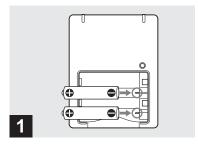
→ Insert Nickel-Metal Hydride batteries into the battery charger (supplied) with the correct polarity +/-.
