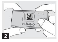
Hold the camera steadily with both hands and position the subject in the center of the LCD screen.
