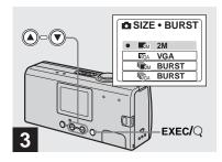
→ Select the desired image size with the control buttons ▲/▼, then press EXEC.
