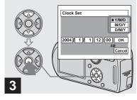
→ Select the desired date display format with A/V on the control button, then press ●.
