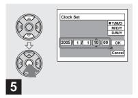
Set the numeric value with ▲/▼ on the control button, then press ● to enter it.
