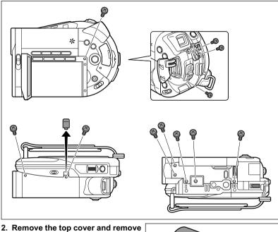
Remove the top cover and remove the additional screws under it.
