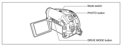
1. Set the camcorder to record still images on the card ( CAMERA · C / @] ) and move the mode switch to a position other than (). If you are recording stills on the disc (), change the media for the still images
