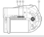
Press the + or - button on the camcorder or the NEXT/PREV. buttons on the wireless controller to move to the next or previous index page, respectively.
