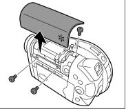
3. Remove the LCD display cover and the back cover.
