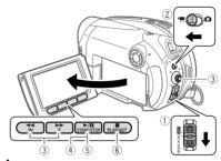
Move the power switch to ON, then slide it down toward MODE and release it to set the camcorder in PLAY mode.
