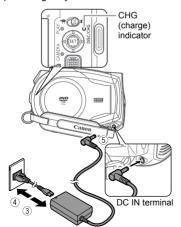
3 Connect the power cord to the compact power adapter.
