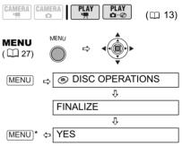
\* During the disc finalization a progress bar is displayed. Close the menu only after the screen display returns to the [DISC OPERATIONS] menu.
