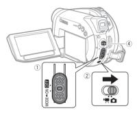
1 Move the power switch to ON, then slide it down towards MODE and release it to set the camcorder in PLAY mode.
