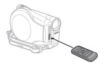
Point the controller at the camcorder's remote sensor when you press the buttons.
