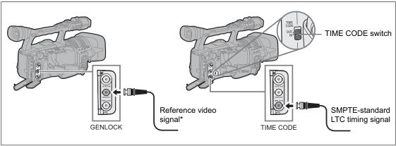
\* As a reference video signal input you can use either an HD Y signal or a PAL composite video signal.
