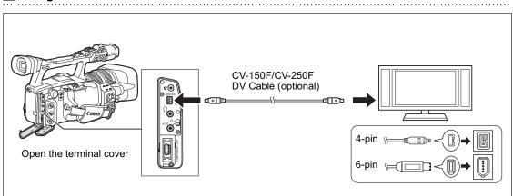
When connecting the camcorder to a monitor TV that supports DV, you may need to carry out a procedure on the TV to recognize the camera. Refer to the instruction manual of the TV or monitor. • If necessary, turn on the DV conversion and select whether to convert a tape recorded in HD to SD with the following procedure.
