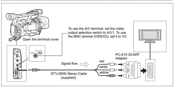
If connecting to a TV set the input selector to VIDEO. If connecting to a VCR, set the input selector to LINE. The supplied PC-A10 SCART Adapter is for output only. For analog line-in recording or analog-digital conversion, use a commercially available SCART adapter with input capability.
