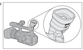
Prevent direct sunlight from getting in the viewfinder. The viewfinder LCD may become damaged due to concentration of the light by the lens. Pay special attention when mounting the camcorder on a tripod, or during its transportation.
