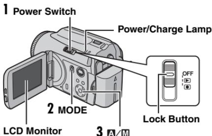
Set the appropriate operation mode according to your preference using the power and **MODE** switches and
