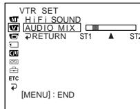
Five minutes after when you disconnect the power source or remove the battery pack, the setting of AUDIO MIX returns to the original sound (ST1) only. The default setting is original sound only.
