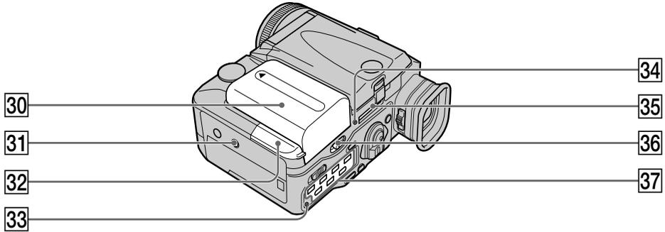
**30** Battery pack/Battery terminal cover (p. 10)
