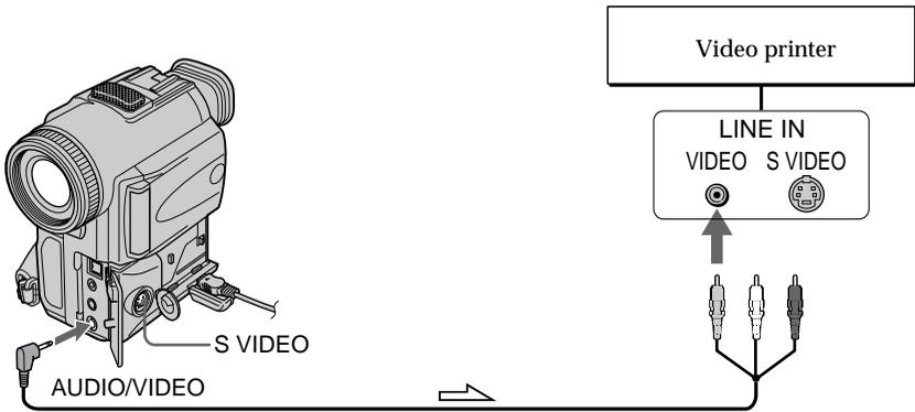
If the video printer is equipped with S video input
