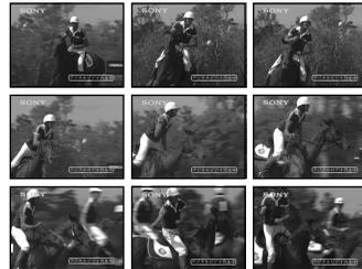
While pressing down PHOTO, the camcorder shoots still pictures continuously. The maximum recordable number of still pictures (1152 × 864: up to four pictures, 640 × 480: up to 16 pictures) is in accordance with the image size setting.
