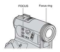
Press FOCUS during recording or in the standby mode.
