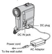
You can charge the battery pack on a trip, even if you have not brought the Handycam Station along. With the ▲ mark on the DC plug facing front, connect the AC Adaptor to the DC IN jack on your camcorder as shown in the illustration.
