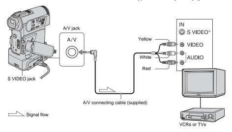
\* By using an S video cable (optional), higher quality DV format pictures can be produced.
