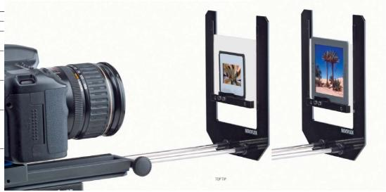
Use a CASTEL-Q focusing rack and Q=BASE mounting plates for transverse camera adjustment. Cameras with a tripod connection on the side can be precisely positioned in this way. This speeds up work enormously when selecting the picture area to be copied because otherwise the whole tripod would have to be set up again.
