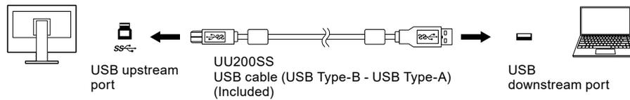
2. Connect a peripheral USB device to the USB downstream port ([page 9](#)) of the monitor.
